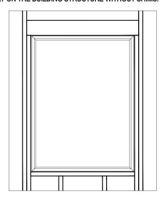
When the unit is tight in the opening, and is square, plumb, and level, use the required fasteners to secure the unit in the opening. Refer to the Shop Drawings for fastener placement. If no drawings were done, make sure the fasteners engage into a structural area of the building with maximum edge distance available.
